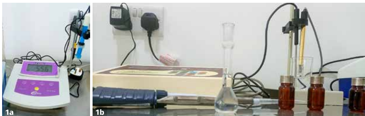
Figure 1 a. pH meter to measure the pH of buffer solutions and eye drops. b. Conductivity meter for water analysis.
